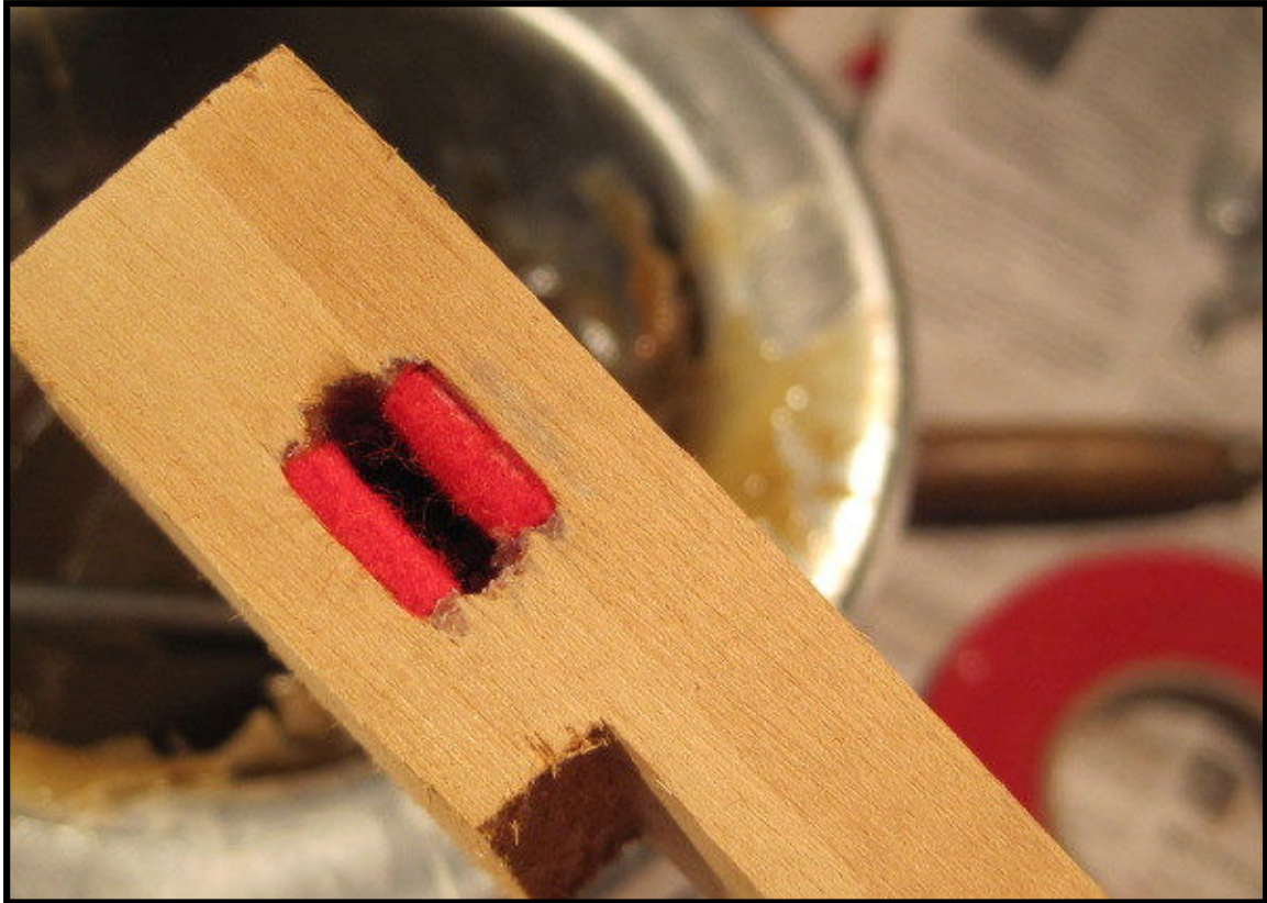
A key which has been professionally rebushed.
